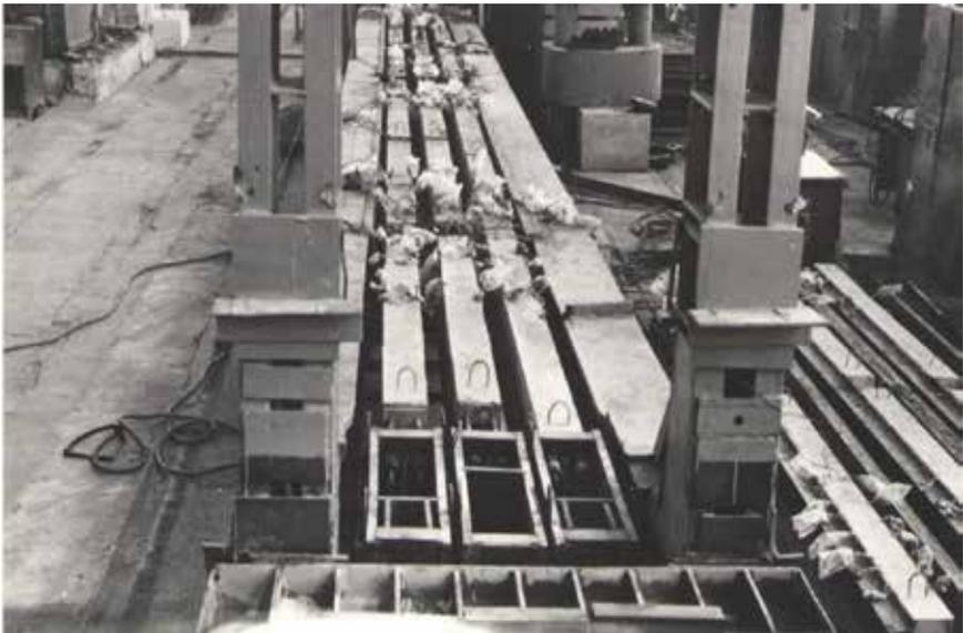
**Fig. 1. General view of prestressed reinforced concrete beams located on the stand and beams without prestressing located outside the stand (see on the right of the stand)**
