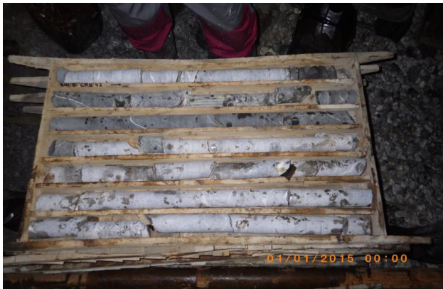
Figure 3 – Defining the RQD indicator a - the procedure for measuring and calculating RQD; б - determination of the RQD index of the Akzhal deposit rock.
